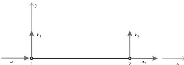
FIGURE 2.3 Degrees of freedom of a rod element in a two-dimensional space.
